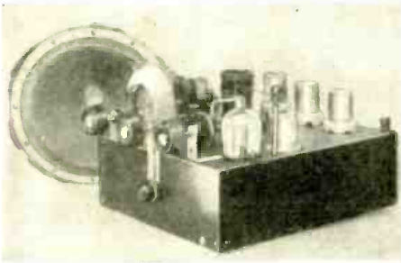
Appearance of Mr. Matthews' 5-meter superheterodyne receiver which employs a single tuning dial; loud speaker appears in the background. The set uses seven tubes in all, including a rectifier.
