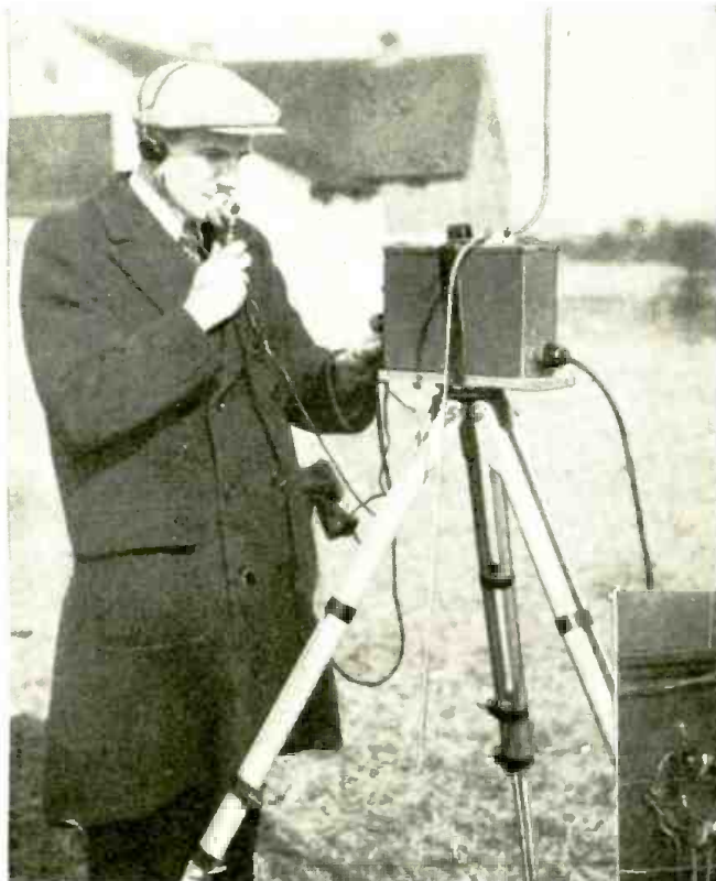
Above—New R. C. A. 5-Meter Transmitter and Receiver. It is "battery-operated" and is thoroughly portable; it can be used in a plane. Its land range is about three miles, but this can be increased by elevating the transmitter.
